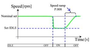
The rotation speed remains set to this value for all the time that the IDLE input remains closed. Opening the IDLE input, the regulator performs a controlled ramp from the Set RPM IDLE (P.004) to the
